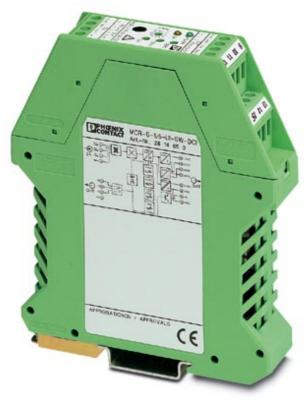
MCR current measuring transducer, programmable and configurable, for measuring direct, alternating and distorted currents, with relay and transistor output, input current 0..0.5 to 0...10 A, unconfigured
